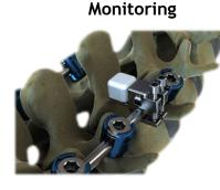
Wireless IoT Strain Sensor
